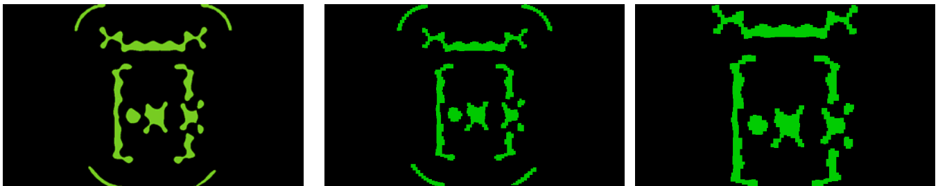
Figure 10a,b,c. Binary masks for SRAM pattern.
