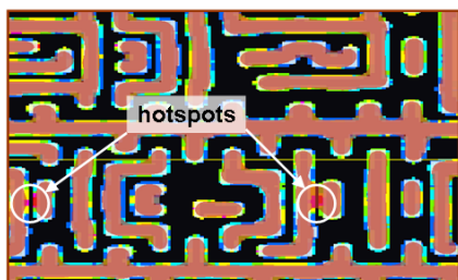
Figure 1c. A 2D metal layout with pixel-based color bitmaps that show random hotspots.
